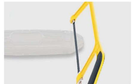
3. select appropriate position for sawing based on requirement.
